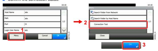
*Connected.* appears when connection to the destination is correctly established. If *Cannot connect.* appears, review the entry.
