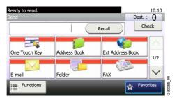
If Program mode is selected, set the copy function, send function, FAX function (option), and destinations to be registered.
