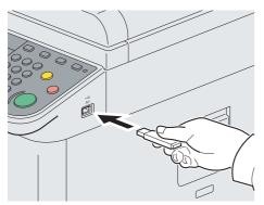
When using USB memory, plug it into the USB memory slot (A1).
