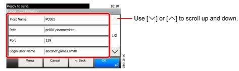
When specifying a computer or server port number as the destination, press [Port] and enter the port number. You can enter a number from 1 to 65,535 with a maximum of 5 digits.
