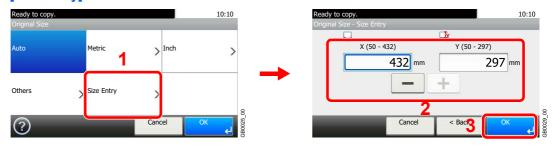
Press the text box displaying the numbers and use [-]/[+] or the numeric keypad to enter a value.
