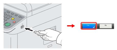
Plug the USB memory into the USB memory slot (A1).
