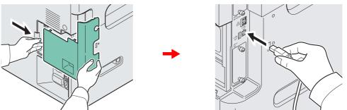
2 Connect the other end of the cable to the PC.
