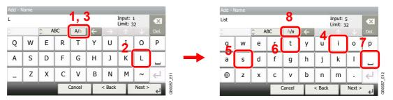
To shift from lower case to upper case letters, press [a/A]. To shift from upper case to lower case letters, press [A/a].
