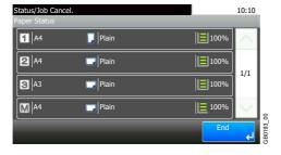
The remaining amount of paper is shown by four levels as 100%, 70%, 30%, and 0% (none), however, the paper in the multi purpose tray is shown by two levels as 100% and 0%. If there is no paper in either cassette, the paper status will be shown as *No Paper*.
