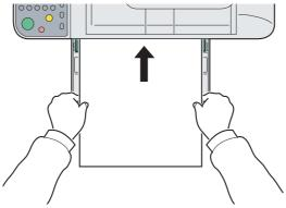
Insert the paper along the paper width guides into the tray until it stops.
