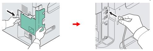
2 Connect the other end of the cable to the hub.
