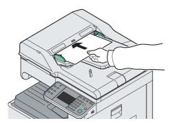
With the side to be scanned face up, insert the leading edge of the original all the way into the document processor. If the original is two-sided, insert with the front side face up.
