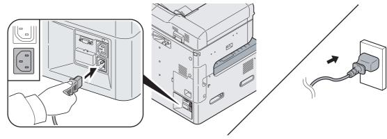
Connect one end of the supplied power cable to the machine and the other end to a power outlet.
