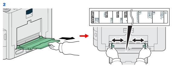
When loading paper sizes from A3 to B4 and Ledger to Legal, extend the support tray section of the multi purpose tray.
