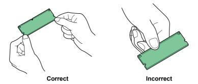
To protect electronic parts, discharge static electricity from your body by touching a water pipe (faucet) or other large metal object before handling the memory module. Or, wear an antistatic wrist strap, if possible, when you install the memory module.
