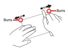
Before loading Hagaki into the multi purpose tray, fan them and align the edges. If the Hagaki paper is curled, straighten it before loading. Printing onto curled Hagaki may cause jams.
