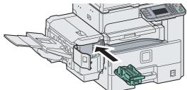
The staple cartridge holder will click into place when it has been inserted correctly.
