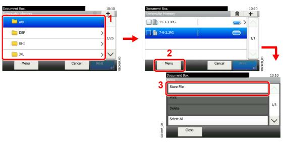
Select the folder where the file will be stored and press [Menu] and then [Store File]. The machine will display the top 3 folder levels, including the root folder. To return to a higher level folder, press [< Back].
