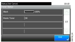
You can check the remaining amount of toner as one of 11 levels from 100 to 0%, and check the status of waste toner box.
