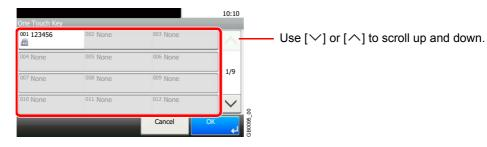
Press the One Touch Keys where the destination is registered. Multiple One Touch Keys can be selected.
