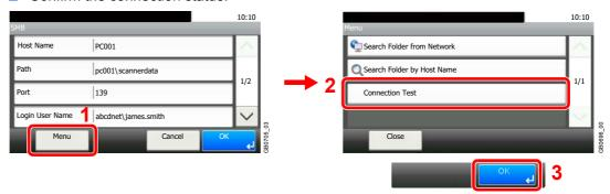
*Connected.* appears when connection to the destination is correctly established. If *Cannot connect.* appears, review the entry.
