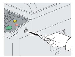
After Removable Memory can be safely removed. is displayed, press [OK] and remove the USB memory.
